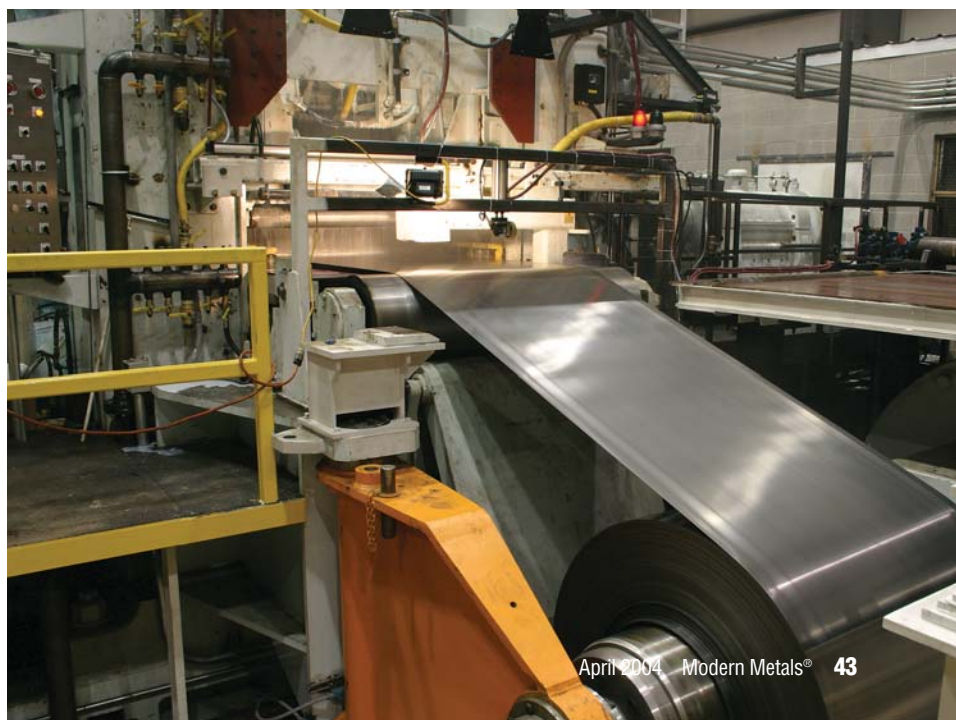
Hydraulic automatic gauge control maintains a \pm 0.0005 -inch thickness tolerance. A complete work- and backup-roll change can be made in 30 minutes.
