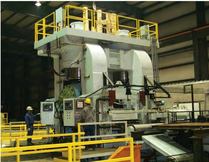
FMP installed a United/Bliss four-high combination reversing cold-rolling mill in 2004 and is in the process of expanding its annealing capacity. Adding cold-roll processing capabilities opened the company up to new customers as its Cleveland market was shrinking. (Photo courtesy Ferrous Metal Processing)
