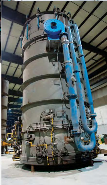
Down in the pit at FMP's Cleveland processing center (top), workers prepare to install new annealing furnaces (above), which will double the company's annealing capacity to 9,000 tons per month. (Photo courtesy Ferrous Metal Processing)
