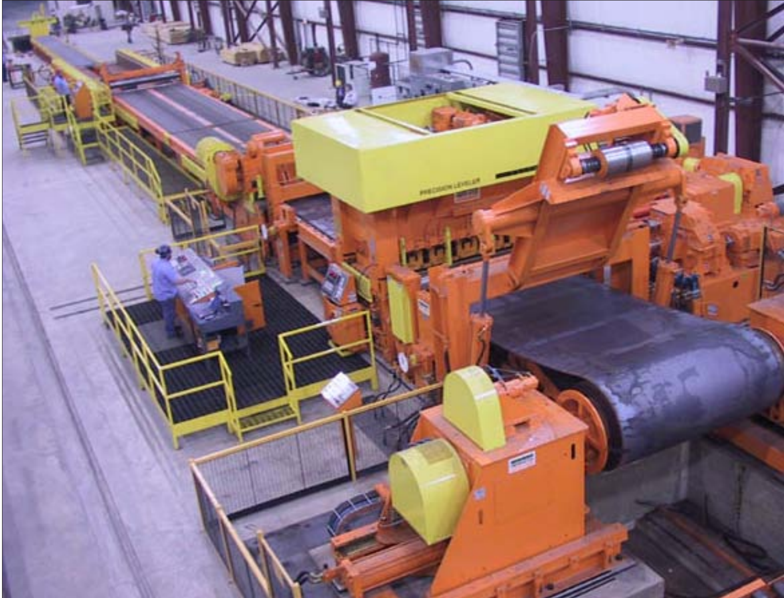
▲ Steel processors may be next in line for a spate of mergers and acquisitions. Shown: A worker at Ferrous Metal Processing, Cleveland, watches master coil enter the leveler.
